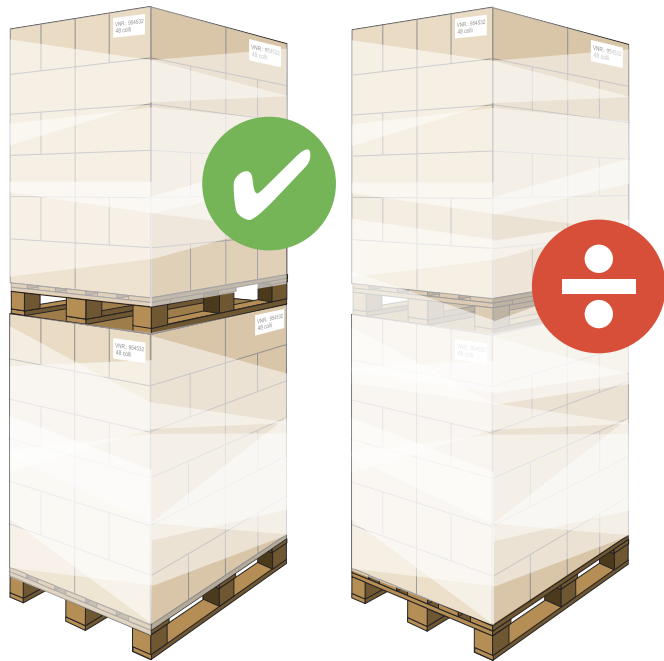
Figure 15: The foil should NOT in any way hinder handling or storage capabilities of the pallet
