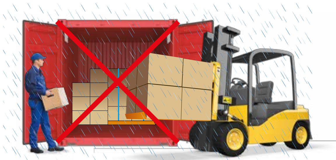
Figure 41: Do not load the container outside when conditions are wet/moist.
