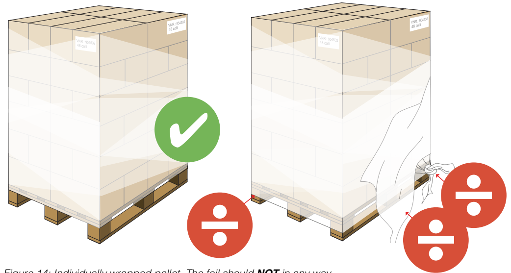
Figure 14: Individually wrapped pallet. The foil should NOT in any way hinder handling or storage capabilities of the pallet .
